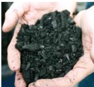
**Biochar produced by Phoenix Energy’s gasification system**
