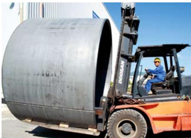
**Colossal:** each of the tower sections weighs up to 60 tons, making a total of up to 250 tons of steel in each tower.
