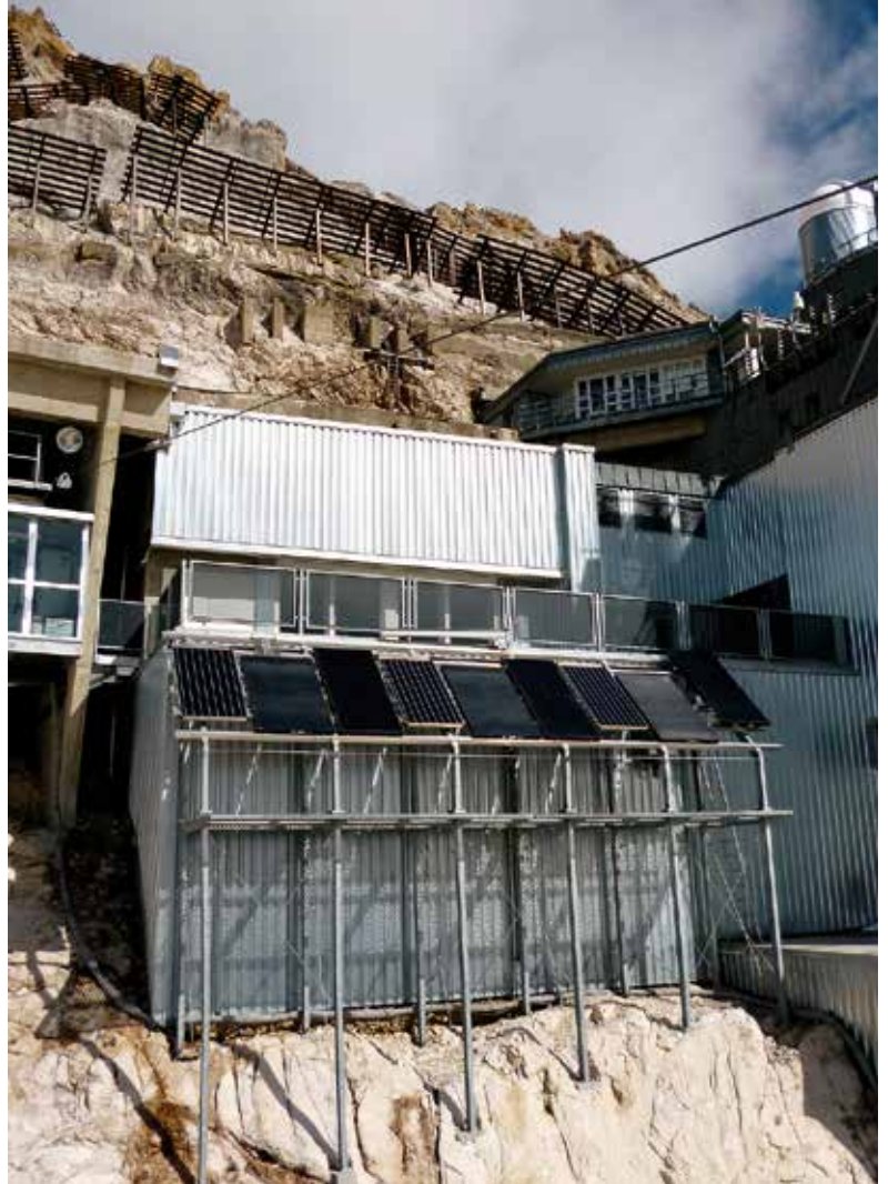
Bracing conditions: At the open-air weather test stand at the Schneefernerhaus on the Zugspitze, the absorber coatings have to withstand extremely high and extremely low temperatures.
